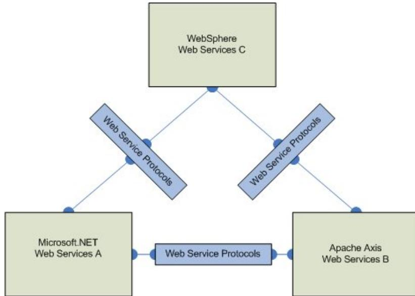
The fact that Application A uses Microsoft.NET on a Windows platform as the infrastructure for its Web Service, while Application C uses Web Sphere on UNIX platform for its Web Service and Application B uses Apache Axis on UNIX platform, is irrelevant. All Web Services still communicate outside of their infrastructure using the same protocols.
